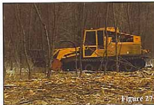
Figure 27 A forestry mower is used to remove non native buckthorn and honeysuckle and restore native prairie areas.
