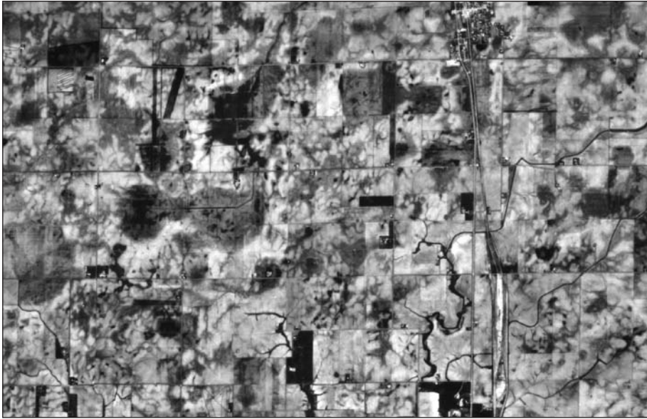
Figure 22 Aerial photograph taken near Clinton in De Witt County, Illinois. The patterned ground surface (mottled surfaces) is typical of that in poorly drained areas where intensive frost action has taken place. Light and dark rectangles and strips are farm fields. (Photograph by W. Hilton Johnson.)
