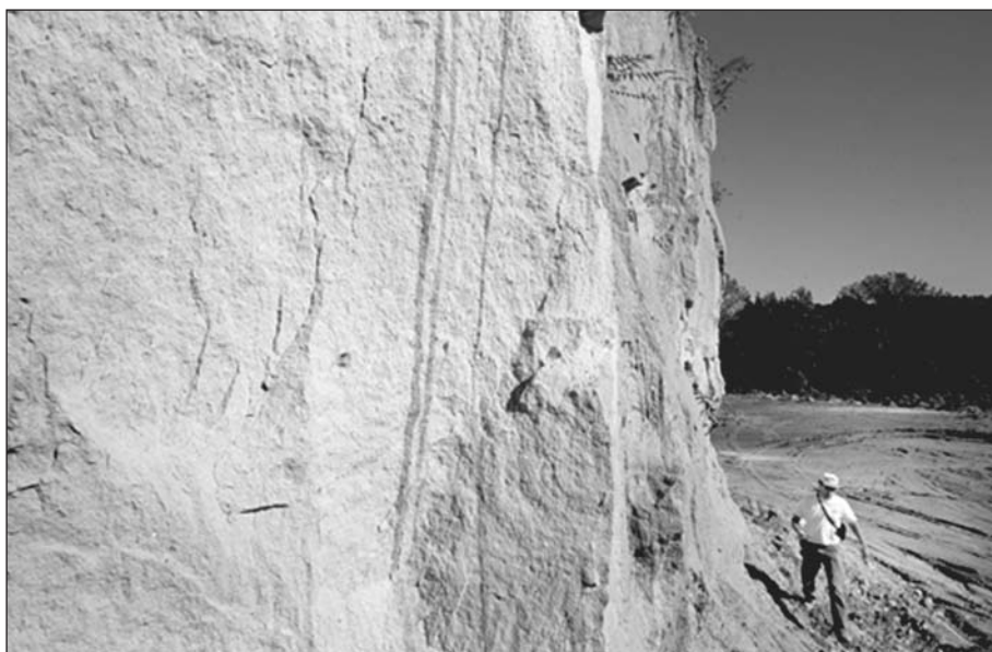
Figure 7 Loess has a uniform grain size and tends to stand in vertical slopes, as shown. (Photograph by Joel M. Dexter.)
